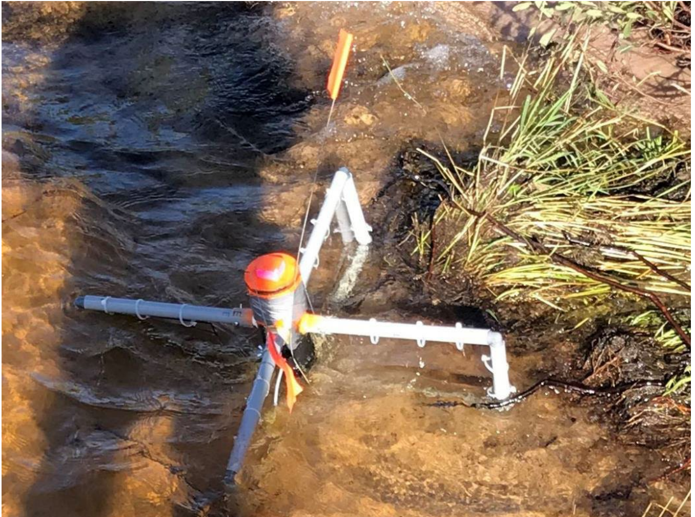
Figure 9: View of a Polyvinyl Chloride Drogue Retrieved after Deployment
