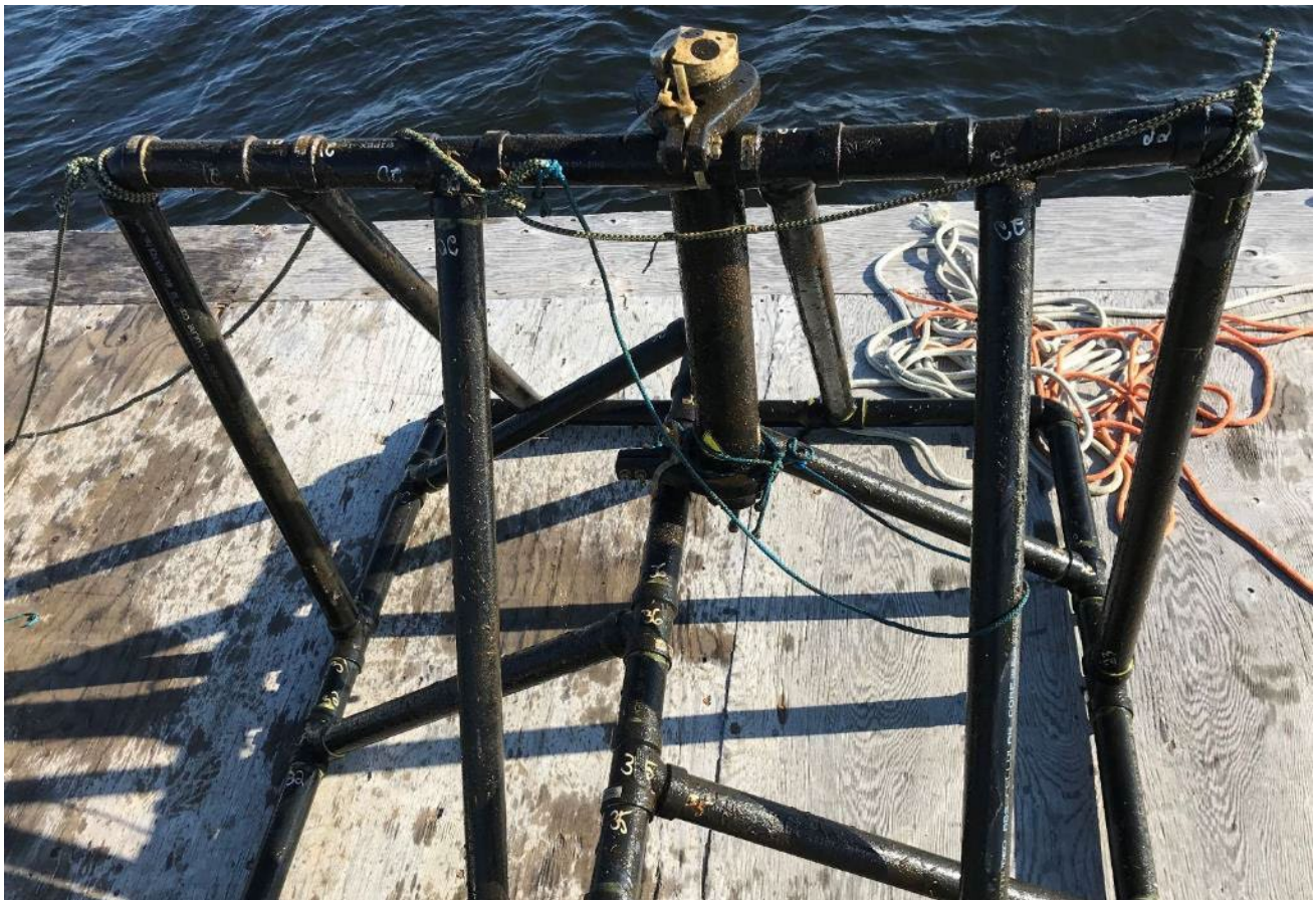
Figure 5: Nortek Aquadopp Acoustic Doppler Current Profiler and Mounting Frame Deployed at Patterson Lake North Intake
