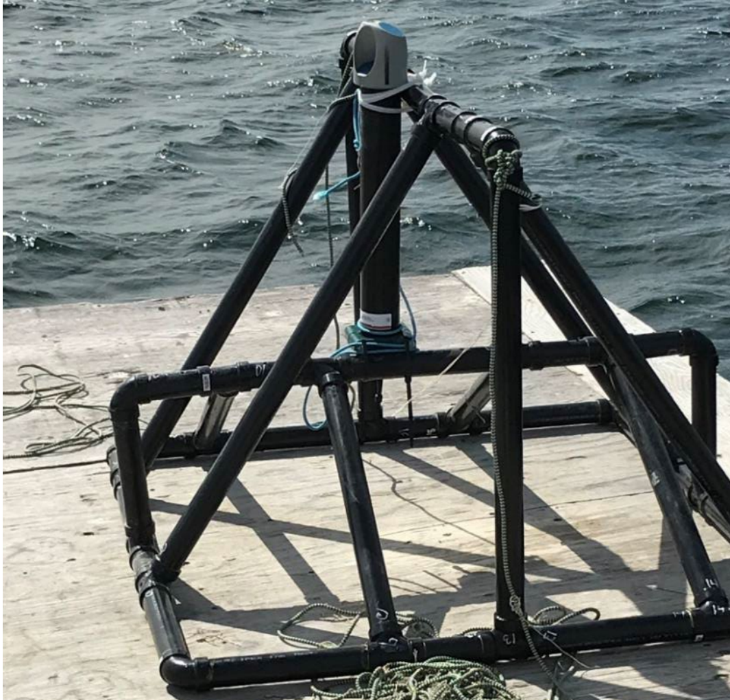
Figure 6: Nortek Aquadopp Acoustic Doppler Current Profiler and Mounting Frame Deployed at Patterson Lake North Outfall
