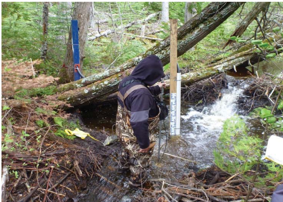
Photograph 8: Manual flow measurements being taken at SPR-HS5 Birch Lake inlet hydrometric station on June 4, 2011; facing east. Installed date.
