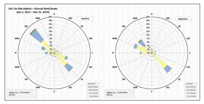
Figure 2-6: Daytime and Nighttime Wind-roses for the CNL On-Site Station Data
