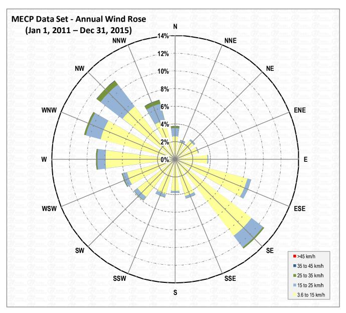
Figure 5-2: MECP Dispersion Meteorology Dataset Wind Rose
