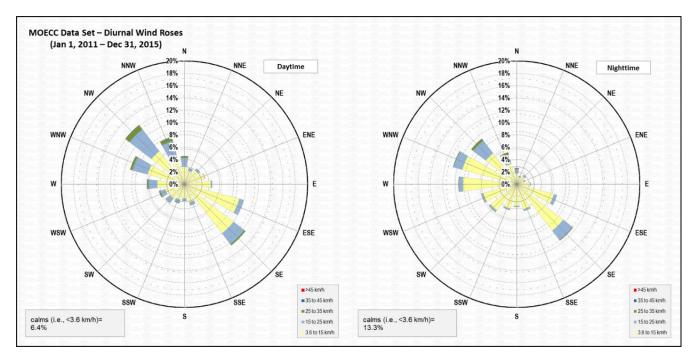
Figure 2-5: Daytime and Nighttime Wind-roses for the MECP Dispersion Meteorology Dataset
