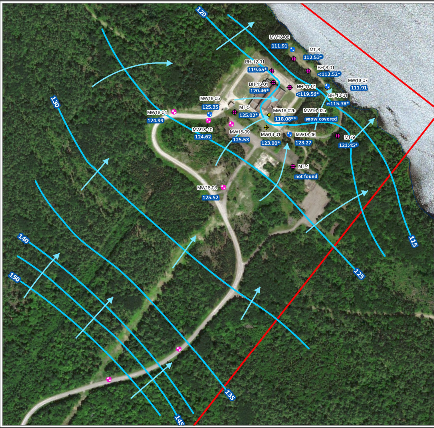
Figure 3.10 Shallow Groundwater Elevations and Flow Directions at NPD Site (January 16, 2018)
