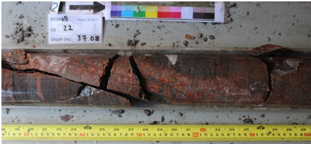
Figure 2.46 Fractured Contact of Subvertical Pegmatite Dyke, BH18-08, 37.5 to 38.1 mBGS
