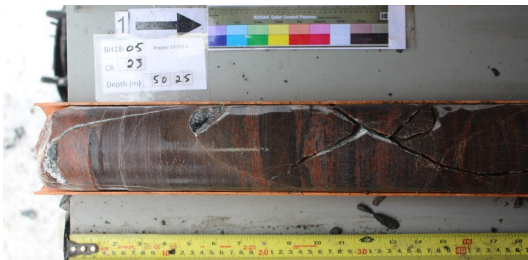
Figure 2.42 Calcite Infilled Subvertical Fractures, BH18-05, 50.2 to 50.7 mBGS
