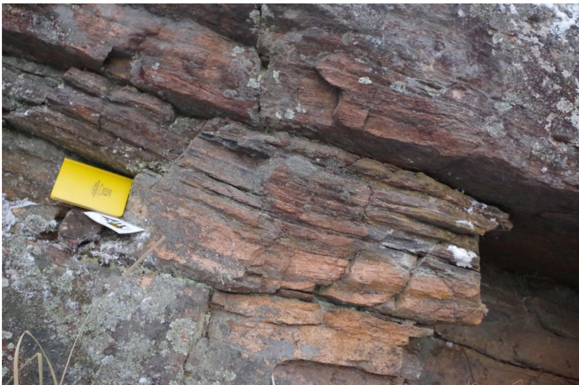
Figure 2.53 Photo 120-5869 – Station 18-NPD-08 – Jointing in Biotite Granitic Gneiss
